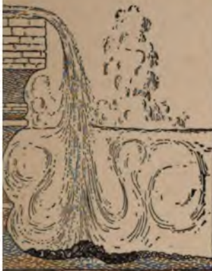
FIG. 380.—Ideal section to show nature of the drilling process beneath the cataract.
